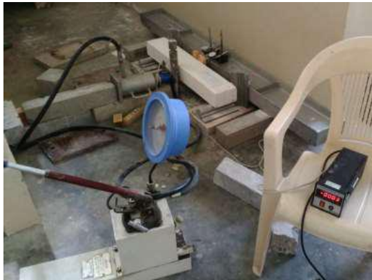
Figure Experimental Set Up for Beam. (Digital Deflect Meter)
